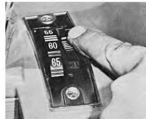
The optional cruise control mounted on cowl can maintain constant speed on either level or hills. A touch of the brake pedal unlocks the system.
