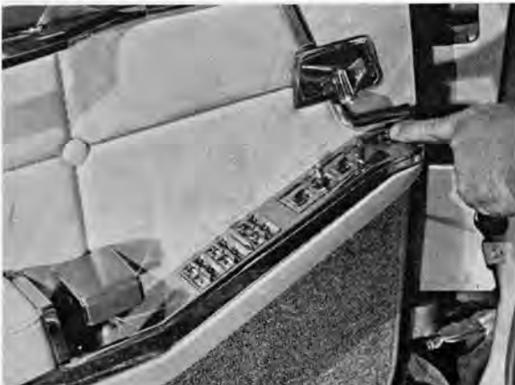
Electric control console on driver's door groups all the switches for windows, windwings, seats, and door locks into one convenient location for fingertip operation.
