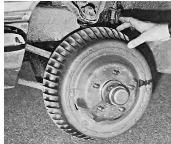
Cast iron drums with cooling fins house self-adjusting shoes. Hydraulic cylinders operated by dual master unit have new long-wearing, sintered-iron pistons.
