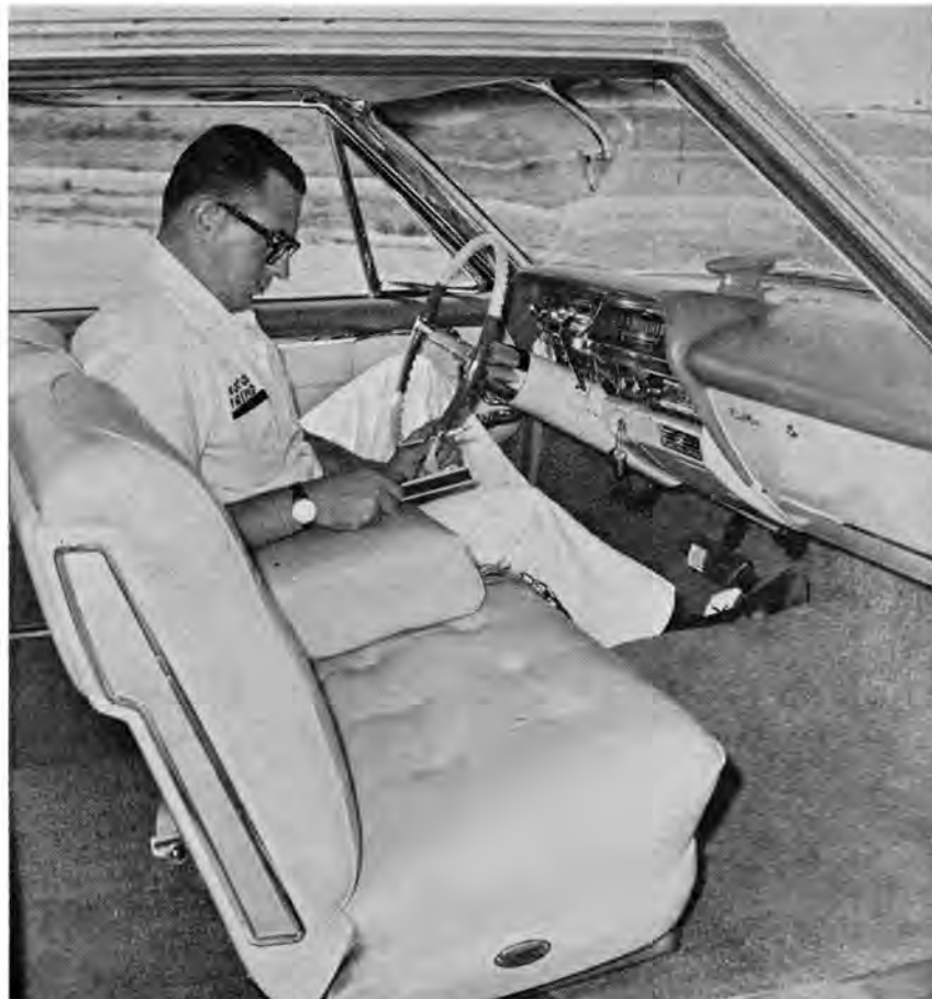
Bench-type front seat (bucket seats are optional) has a center folding arm rest, well padded and wide enough for both driver and passenger. Both front seat backs can be tilted forward for easy rear seat access.
