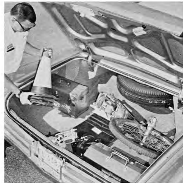
More usable luggage space is available through location of spare in seldom-used area over the rear axle body hump.
