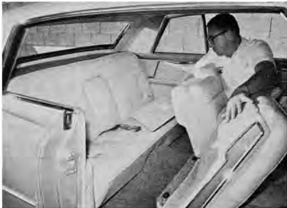
Rear seat has a folding center arm rest that doesn't interfere with the center seat back comfort when stowed.
