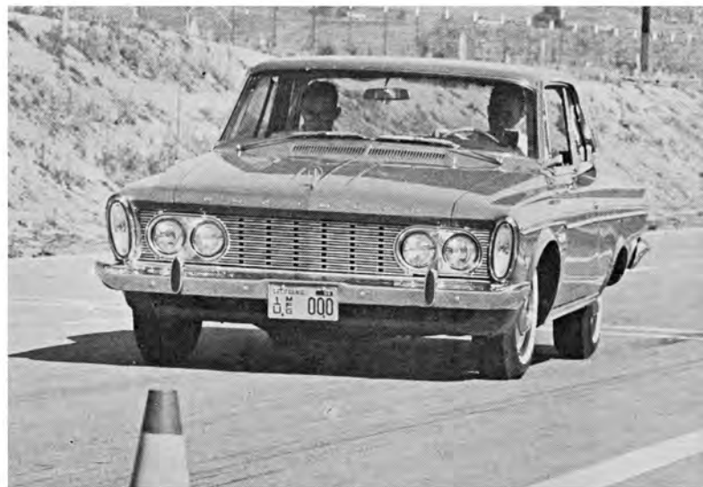
Rear springs, while behaving perfectly under acceleration, let rear wheels hop during panic stops, and caused some swerve.
