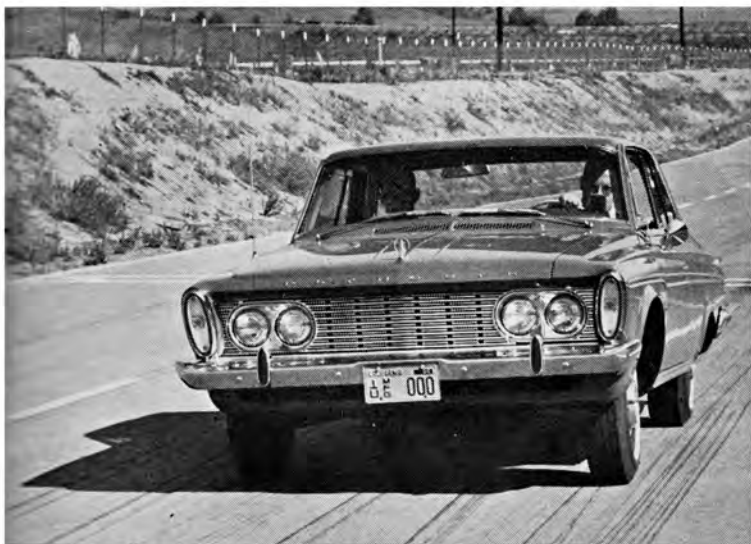
Under hard acceleration, Sport Fury exhibits nose-high stance that shifts the weight back in the direction of the rear wheels.
