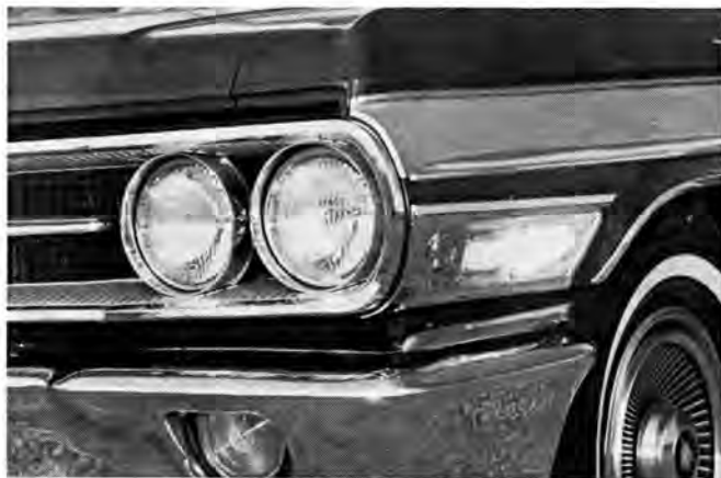
Turning into darkened streets or driveways is made easier with this turning light. It switches on with the turn indicator.
