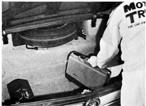
Very few cars can offer any more usable trunk area than this. Drawbacks are hard-to-reach spare and a high lip.
