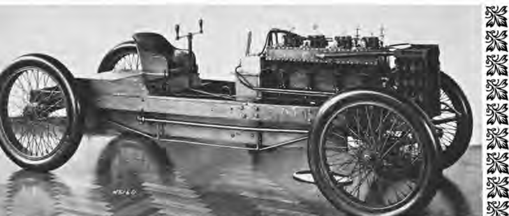
Restored to semi-original form and now resting in the Ford Museum, "999" has radiator from Oldfield period, atmospheric inlets from earlier era. Frame is metal over wood.
