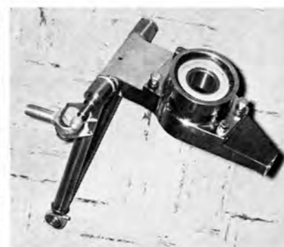
(LEFT) Light alloy bearing carriers are part of adjustable, independent rear suspension system.
