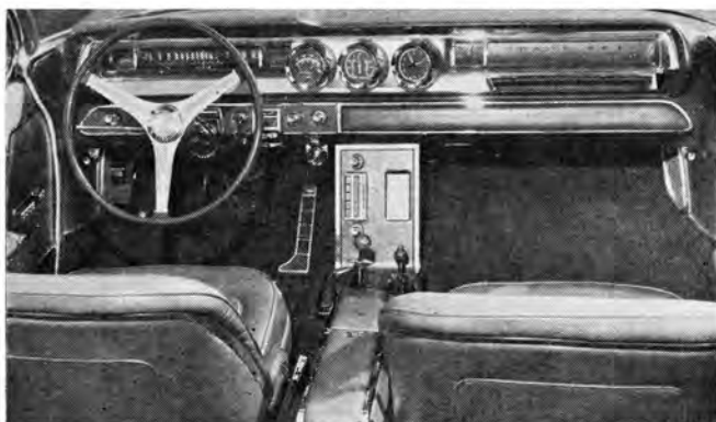
Wood-rimmed wheel and angled instruments are a nice touch. Lever to right of shift lever controls loudness of exhausts.
