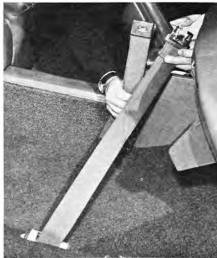
Seat belts are carried in a spring-loaded reel. An internal inertia brake keeps them from extending suddenly on impact.
