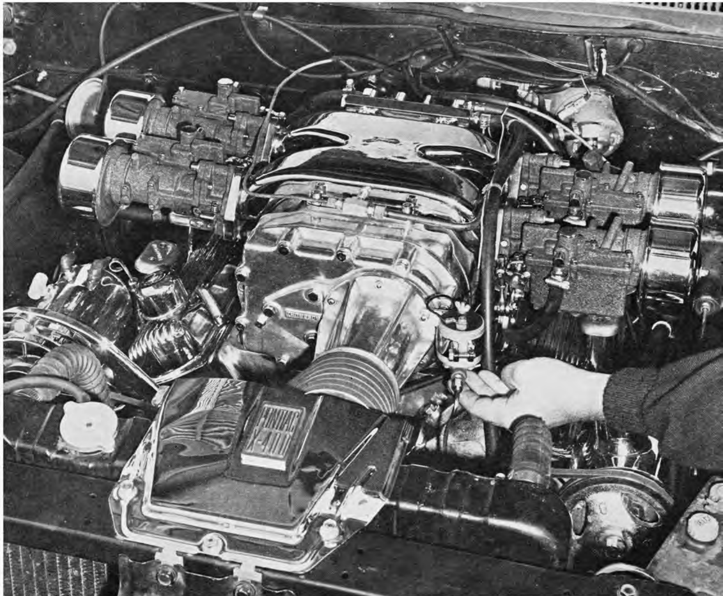
Electric-starting carburetor ensures easy starts when engine is cold. Although boost is limited to 5½ psi, the Thompson-
