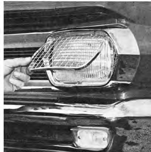
Headlights are protected by wire grilles that swing up to allow cleaning. Novel oblong lights have single bulb elements.
