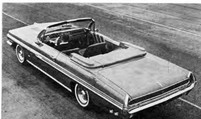
Exhaust pipes are routed through each rear fender. Note the fiberglass top boot and twin, bullet-shaped side-view mirrors.
