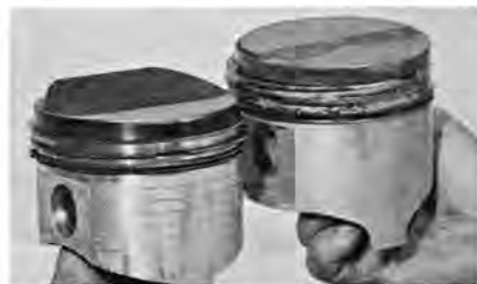
Mickey Thompson 13.5-to-1 forged pistons (left) were used instead of stock units.
