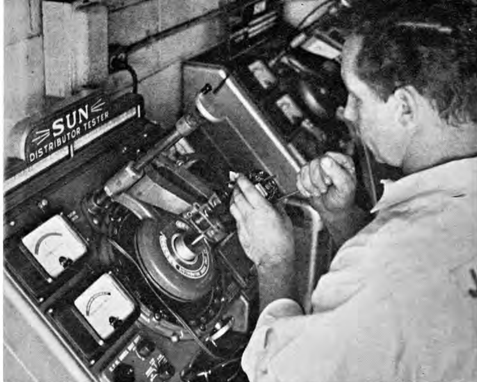
Advance curve of stock "413" distributor was changed slightly to meet the needs of this particular engine. Slight point bounce was cured with sponge rubber pieces.
