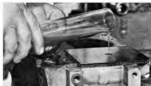
We checked combustion chambers for volume, reduced them to allowable minimum by milling heads.
