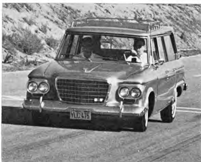
(ABOVE) Nose-dive tendency was a bit pronounced, but all stops were made in a minimum distance, with everything under control.
