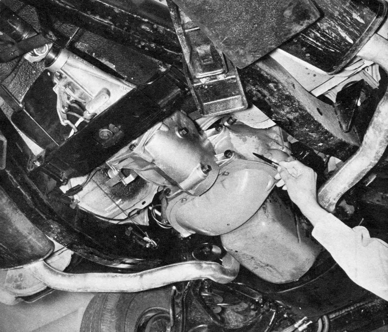
Among production line components advantageous to high performance minded enthusiasts is aluminum transmission case.
