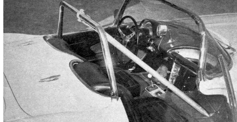
Either full-cockpit or hairpin type of roll bar serves on Corvette. At left is Moon removable type; at right, permanent custom job.
