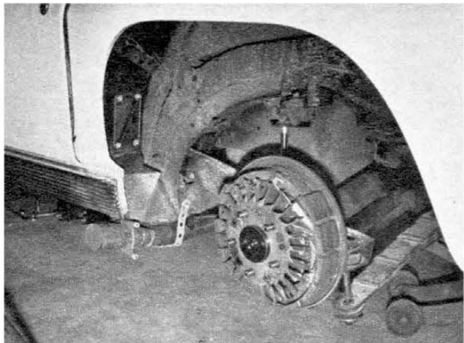
Cooling fan blades must be bent to provide proper clearance.
