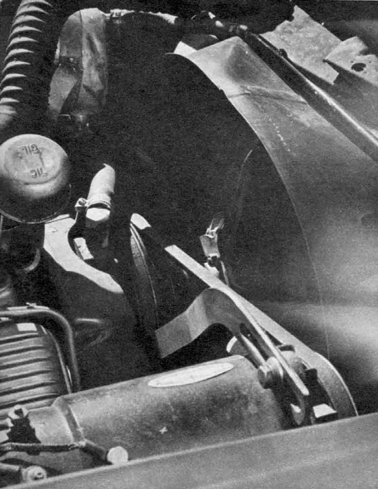
Correct alignment of pulleys and fan belt tension is required.
