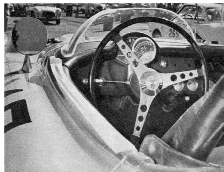
ABOVE—Surplus plexiglas bubble was formed into neat racing screen for this Corvette. ABOVE RIGHT—Full wrap-around type was made from sheets of lucite. RIGHT—Many drivers prefer electric tachometer mounted directly ahead. BELOW—The window post has been cut, but it can be removed easily.
