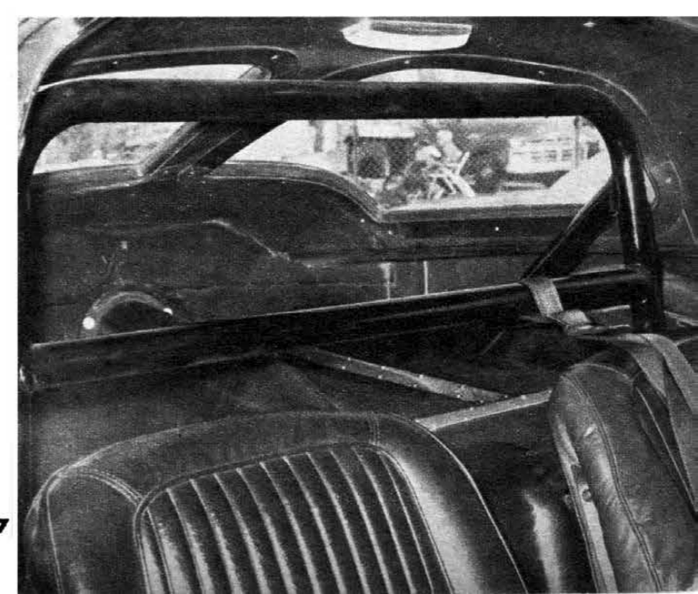
Installation diagram of Moon roll bar reveals simplicity, strength of arrangement. Stands at bottom remain in car.
