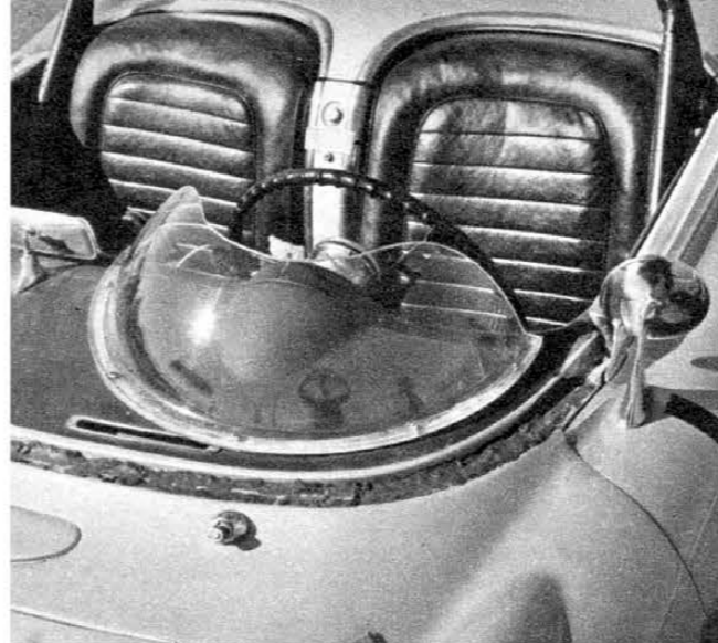
ABOVE—Surplus plexiglas bubble was formed into neat racing screen for this Corvette. ABOVE RIGHT—Full wrap-around type was made from sheets of lucite. RIGHT—Many drivers prefer electric tachometer mounted directly ahead. BELOW—The window post has been cut, but it can be removed easily.
