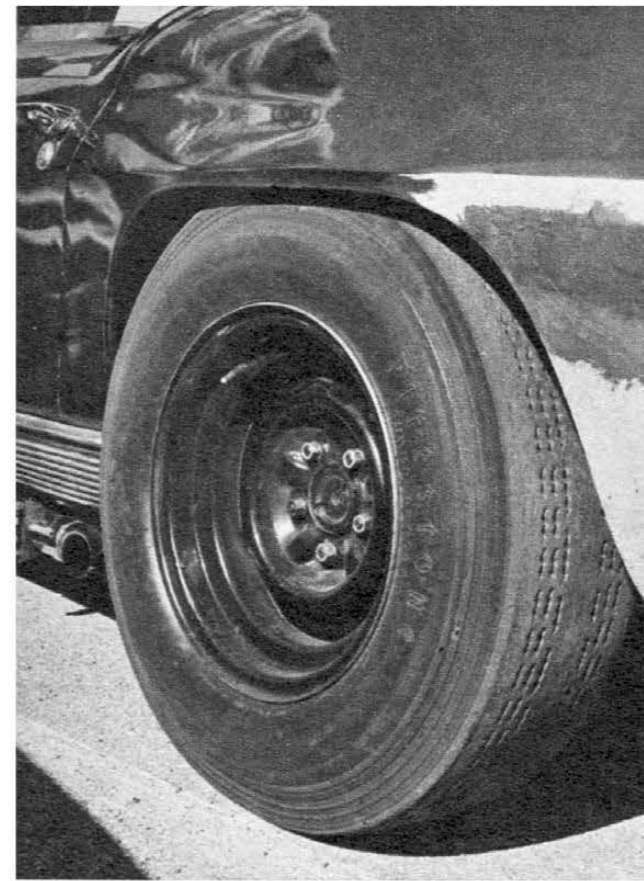
ABOVE—The rear bumper should be removed, and brackets, if possible. LEFT—Wide base rims and special racing tires are a big contribution. BELOW—Properly prepared Corvette, as it is seen by a good many competitors on the road racing circuits.
