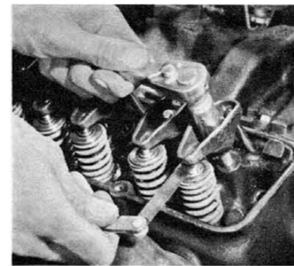
LEFT: Importance of correct valve stem-rocker arm clearance cannot be overstressed. Delicate touch with feeler gauge or use of dial indicator gage is necessary.
