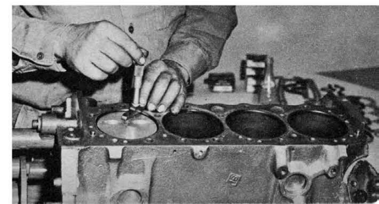
BELOW: Use of a number of precision measuring devices is necessary. Deck height of piston is checked by micrometer.
