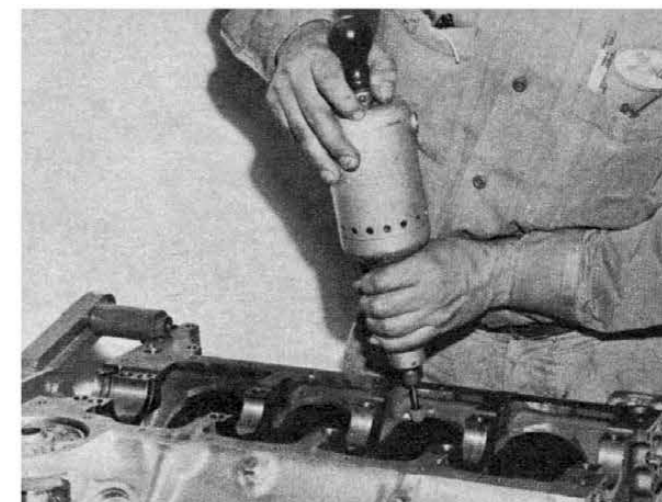
Increased stroke often calls for notching Chevy block. Hand porting tool is being used here to establish clearance for larger counterweight of stroked crank. This does not reduce strength.
