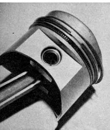
Full floating wrist pins are common practice, make piston changing easier, decrease drag. 409 crankshaft has longer counterweights, will not fit in 348 block without alterations.
