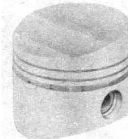
After 409 block is bored to .060 inch maximum allowed by NHRA it is honed by hand. Special pistons for 409, designed to improve combustion chamber shape, are offered.
