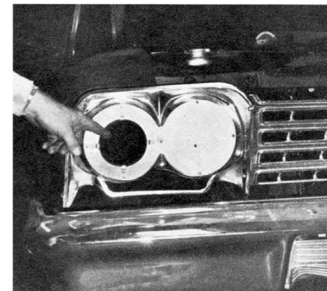
Source of cooling air for brakes is spot ordinarily occupied by outboard headlight. Lights should be removed for competition.
