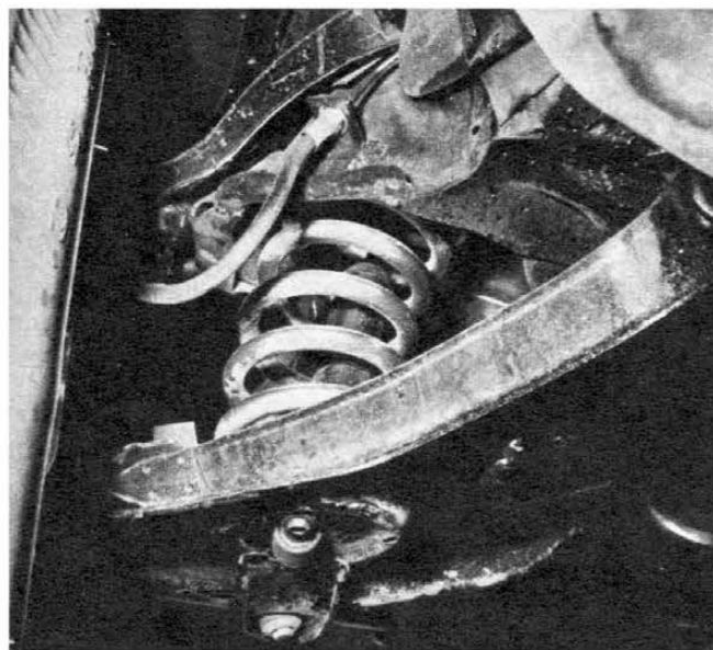
RPO 1108, Chevy optional suspension kit for Police cars and off-the-road service includes stiff front coil springs shown here.
