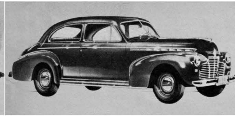
1941 Chevrolet was tremendous pre-war "street" favorite of hot rodders because of its clean lines and an improved engine, rated at 90 bhp. Speed equipment became available for this engine, but the later 235 "Powerglide" engine received bulk of hop up treatment and attention from serious hot rodders.
