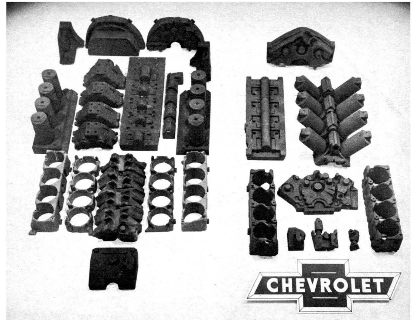
Small number of separate foundry cores used in Chev V8 (right) helps keep tolerances close, production costs down. RIGHT: Bell housing adds to stiffness of block. BELOW: Five head studs in pattern around cylinder instead of conventional four, aids head-block sealing.
