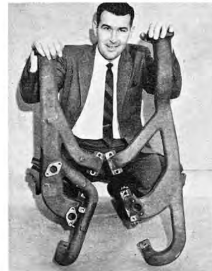
Divider wall between intake ports extends part way up manifold passages. Balance pipe dimensions are critical for performance.
