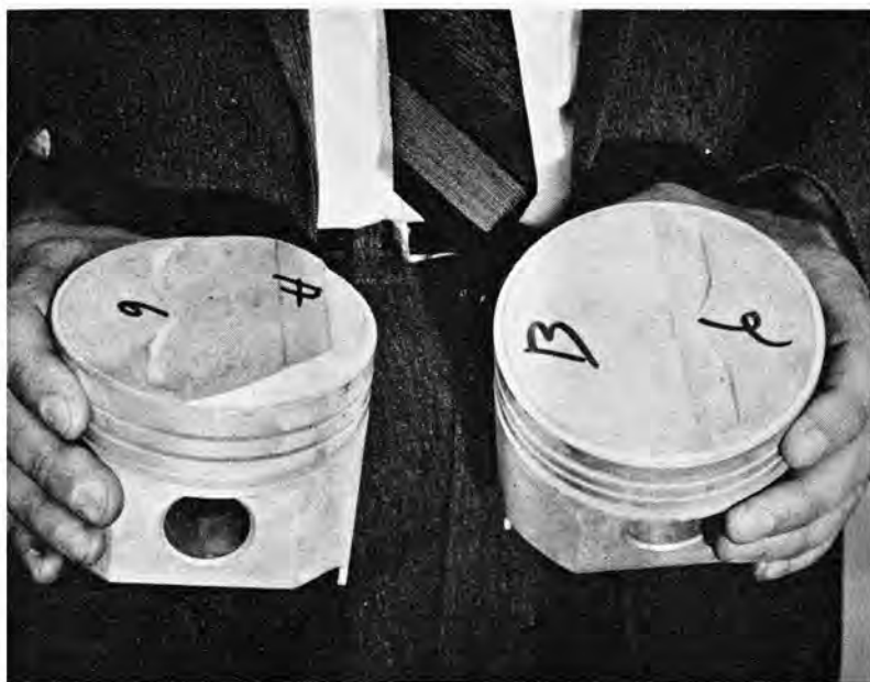
13.5 pop-up piston, left, is shown with J's flat piston. The 9.6 J piston has been given eye-brows in order to gain extra valve clearance.
