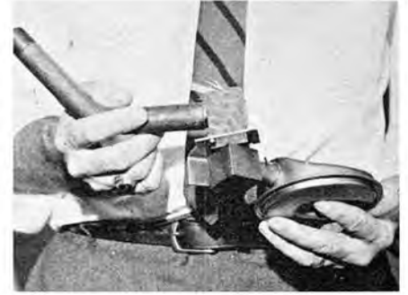
Oil pickup line was increased to 9/16-in. inside diameter. Swivel is bigger. Float swings sideways.
