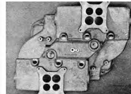
Top of 426 Short Ram intake is shown for comparison. It was designed for power in the top rpm range.
