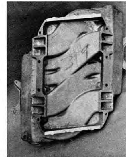
Long exhaust manifold branches help separate individual pulses, prevent exhaust overheat interference between adjacent cylinders.
