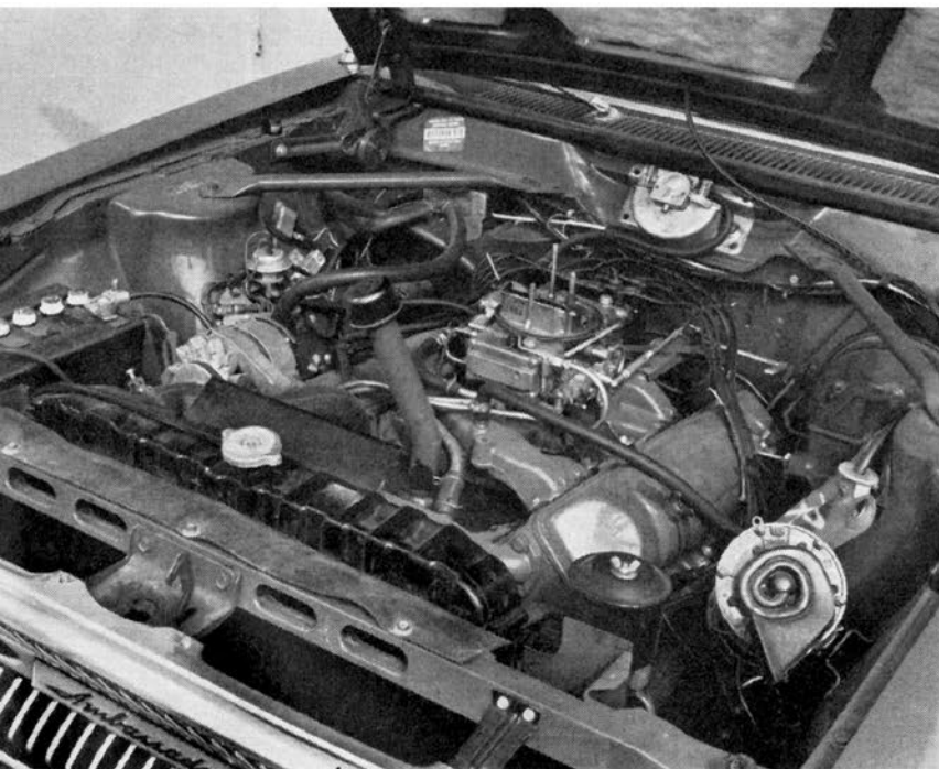
4-BARREL CARBURETOR , dual exhaust system help promote 270 bhp.
