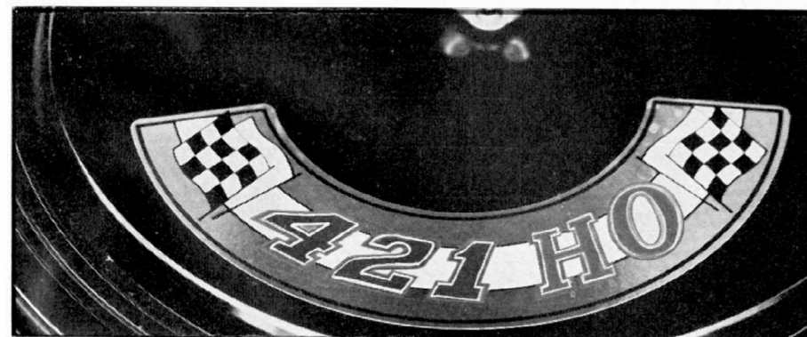
LABEL ON THE aircleaner cover identifies the 421-cu. in. High Output engine option.
