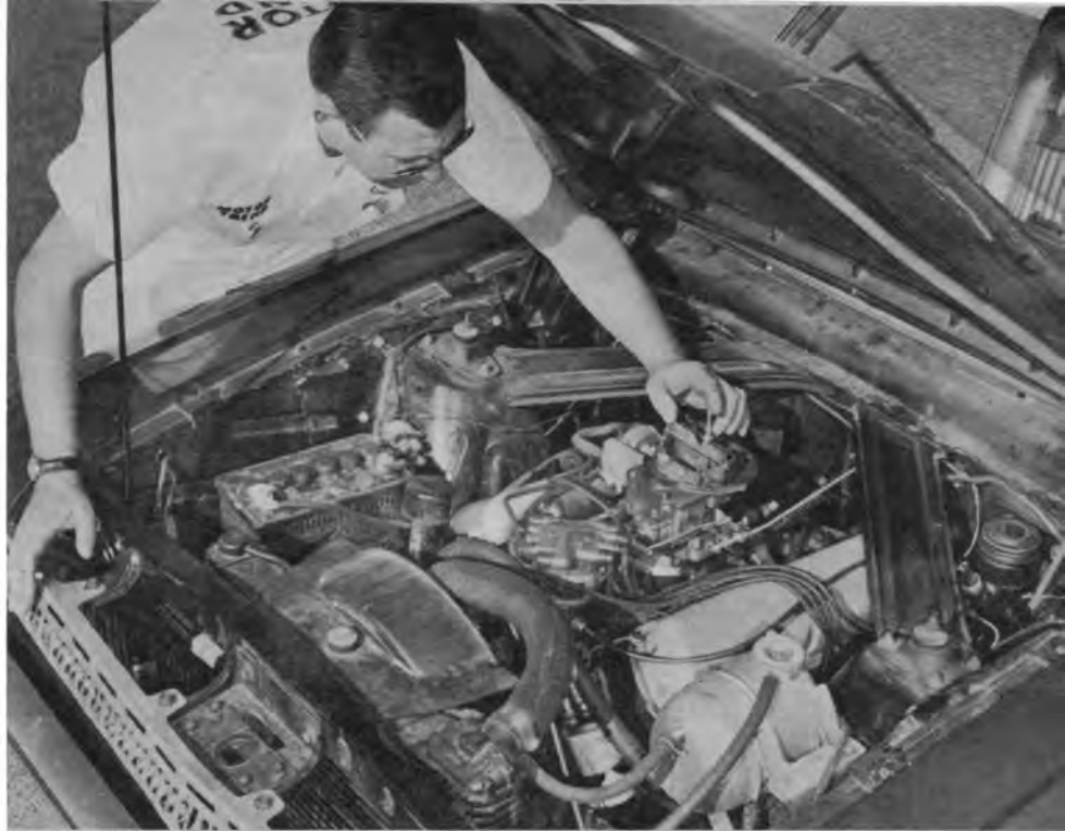
The "260" fits nicely in the Falcon's engine compartment. There would have been even more room if the body hadn't been sectioned three inches. Lightweight, efficient Airheart discs (left) are used on all four wheels to provide quick, fade-free stops.
