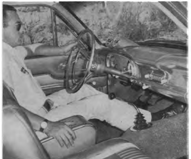
Aluminum plate blanks off unused stock speedometer, while boat-type housings hold Stewart-Warner tachometer and speedometer.
