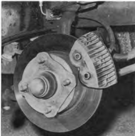
The "260" fits nicely in the Falcon's engine compartment. There would have been even more room if the body hadn't been sectioned three inches. Lightweight, efficient Airheart discs (left) are used on all four wheels to provide quick, fade-free stops.
