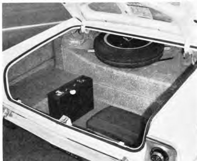
Trunk sill is low enough to avoid interfering with loading procedures, and with spare out of way, usable area is plentiful.
