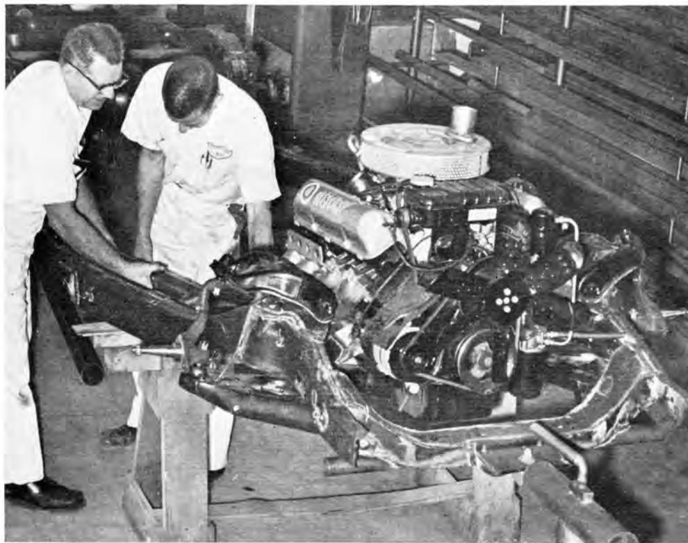
(ABOVE) Mercurys are prepared for racing at Bill Stroppe's shop. Here technicians fit exhaust system through side of frame rail.
