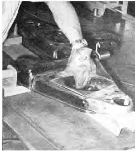
Racing Mercurys get alterations that contribute to safety but not to performance. One such is rebuilding the front A-arms.
