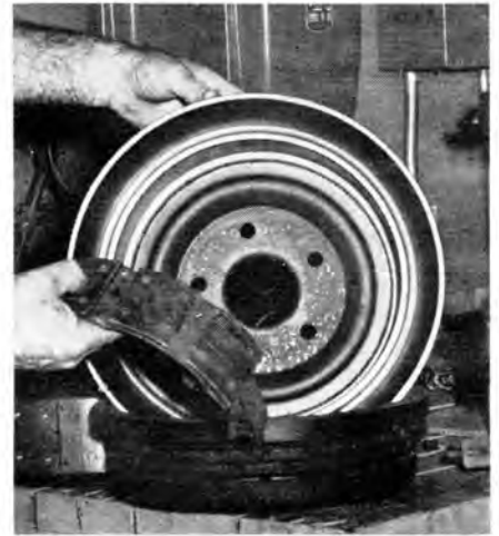
Standard Mercury brakes are not quite up to racing, so Lincoln drums with cooling bells are substituted. Lining is metallic.
