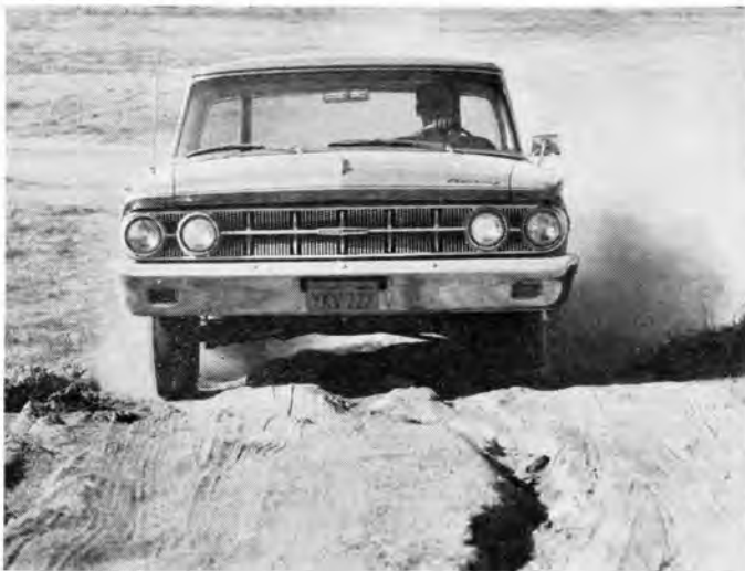
THE MERC HANDLES WELL ON ROUGH ROADS AT SPEED, BUT UNDERSTEER IS EXCESSIVE IN TURNS. ROLL ISN'T AS BAD AS IT FEELS.
