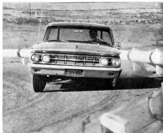
THE MERC HANDLES WELL ON ROUGH ROADS AT SPEED, BUT UNDERSTEER IS EXCESSIVE IN TURNS. ROLL ISN'T AS BAD AS IT FEELS.
