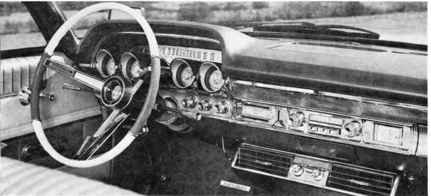
BACK BY POPULAR DEMAND IS A FULL ARRAY OF REAL GAUGES, ALL EASY TO READ AND INDIVIDUALLY HOODED TO PREVENT UNWANTED GLARE.
