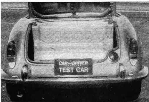
Luggage space is unobstructed; 12½-gallon fuel tank is hidden below trunk floor.
