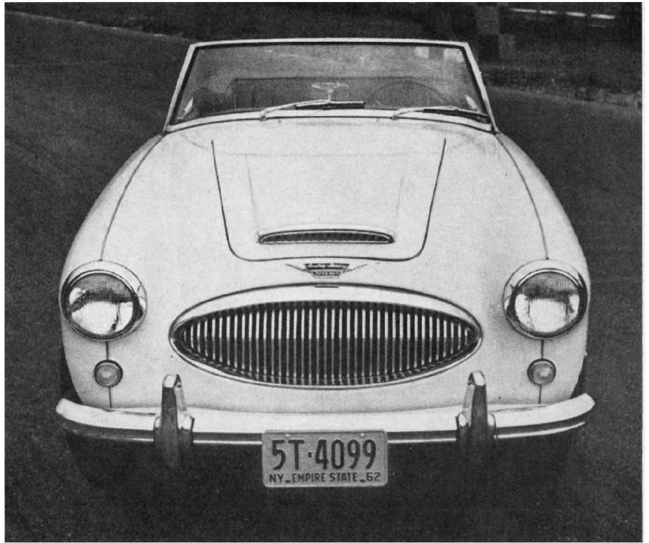
A long hood covers the powerful six-cylinder engine, which is set well back in the chassis. The forward slope provides a good view from behind steering wheel.
