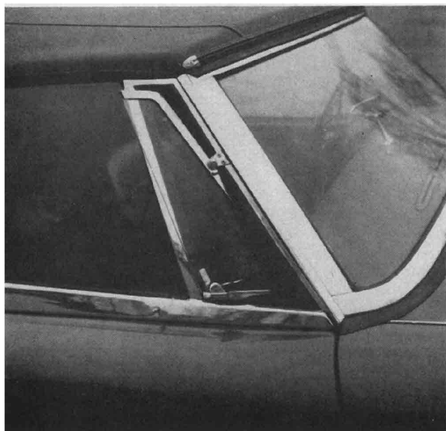
Roll-up windows and vent panes! Creature comfort and convenience come to the traditional sports car, English style.
