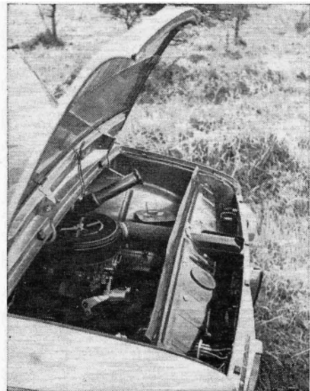
Neat engine compartment offers good accessibility. Hood locks from outside.
