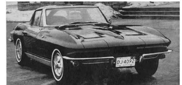
Directional and parking lights are part of bumper design but the retractable headlamps are concealed for daytime driving.
