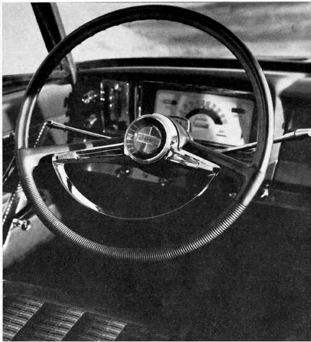
POWER STEERING and a pleasant easy-to-read instrument panel help make the Wagoneer a comfortable car. Automatic transmission indicator quadrant is on steering column.
