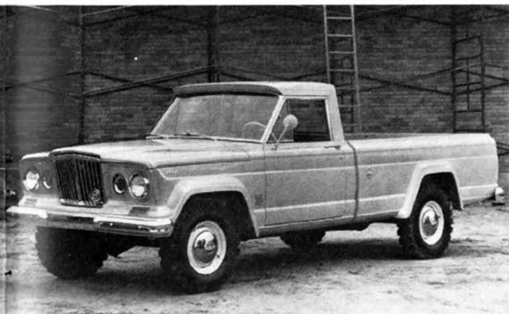
GLADIATOR VERSION (left) of new J Series utilizes many of the same body panels as the Wagoneer, offers the same power and suspension options.
