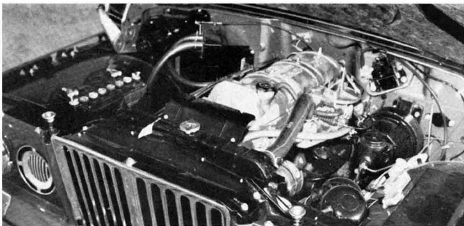
POWERPLANT IS Willys' new Tornado overhead cam 6-cyl. Note accessible location of spark plugs. Engine compartment is big enough to allow easy service.
