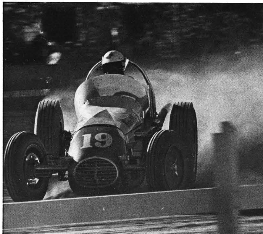
DIRT TRACK racer "broadsliding" around turn is classic oversteer study.
