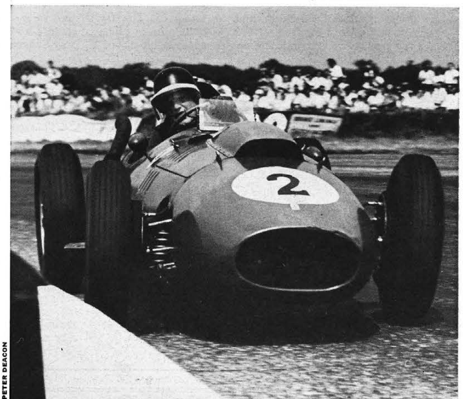
FRONT WHEELS turning hard into corner indicate Ferrari basically understeers.
