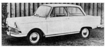
**DKW** Auto Union, a member of the Daimler-Benz group, recently introduced a much-improved version of the DKW Junior. Called the DKW F-12, its three-cylinder, two-stroke engine displaces 900cc, produces 45 hp, and pushes the car to 83 mph. It seats four, drives through the front wheels.
