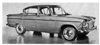
Humber This 1.6-liter Humber Sceptre, built on basically the same unit body as the Hillman Super Minx and Sunbeam Vogue, has an 85.5-hp Four, disc brakes on the front wheels, and overdrive in third and high. The windshield is compound-curved, running into the front of the roof.
