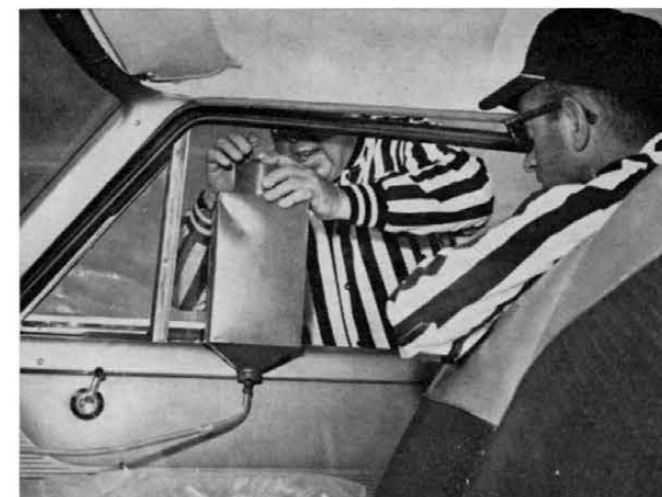
NASCAR officials install pre-measured gallon of pump gas for economy section of tests. Distance must be traveled within a minimum time limit and includes several stops and starts.
