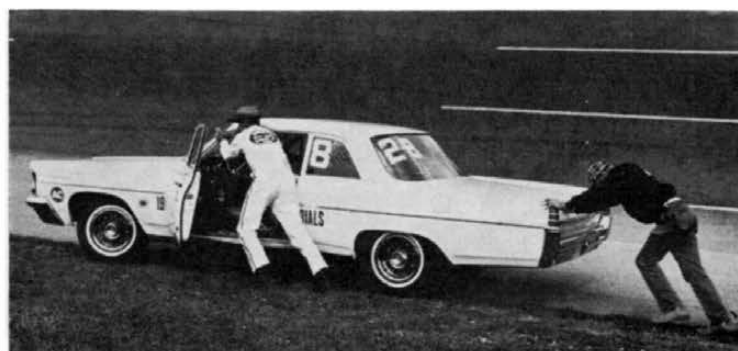
Completely out of fuel, driver Smokey Yunick pushes Pontiac Catalina off the course after clocking 18.123 mpg with big 421-cubic-inch V-8.
