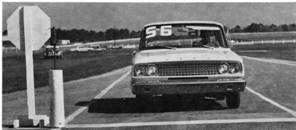
Maximum-effort stops were judged on the basis of total braking distance and the ability of the car to remain within the limits of its designated traffic lane. Fifth wheel distance-measuring device was actuated by brake pedal, recorded tenths of feet.
