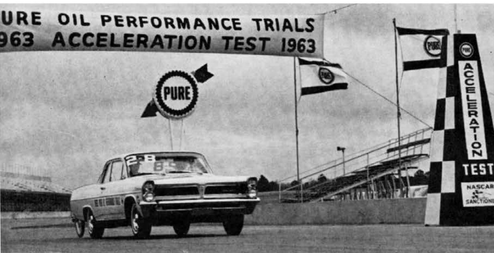
Pontiac Catalina, driven by Smokey Yunick, nears the end of the 25-to-70-mph test for passing-speed acceleration, winning this phase for Class II cars at 6.199 seconds.
