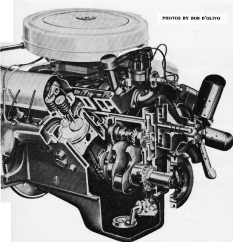
Well proven 390-cubic-inch engine, borrowed from the Thunderbird, is rated at 300 horsepower. Another variation of this engine (Police Performance) uses different camshaft to produce 330 hp.
