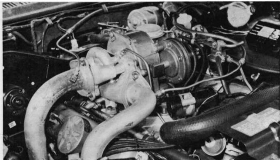
Griffin's Jetfire has gauges to show pressure between the carburetor and the blower.
