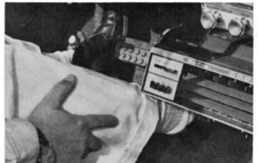
(ABOVE) Air conditioner's location interferes with leg room, could hinder driver's foot in emergency stop. Position changes are planned.
