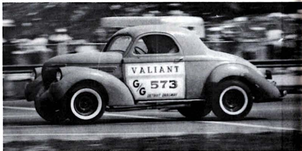
Older cars of the 1930's are extremely popular Gas Coupes. Models such as the '37 Willys (above) and '35 Plymouth (below) are sought because of their relatively short wheelbases and high centers of gravity.
