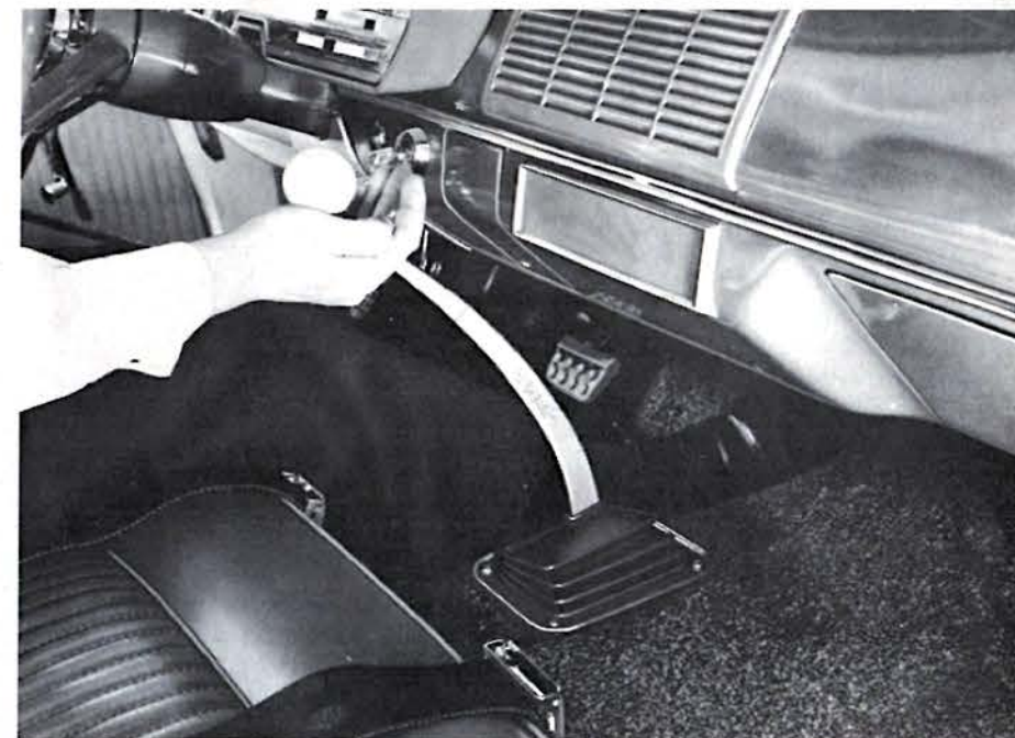
Borg-Warner four-speed manual transmission is available in the '63 Dodges. Standard with this transmission is the Hurst-Campbell floor-mounted shift.
