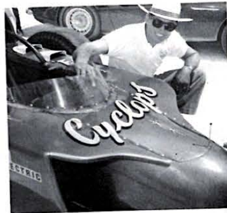
Art Arfons Cyclops turned on at Bonneville to the tune of 338.79 mph. Airfoil on top of car was used to hold it down. Unique sighting device on front of nose gave driver warning in case the car became airborne.
