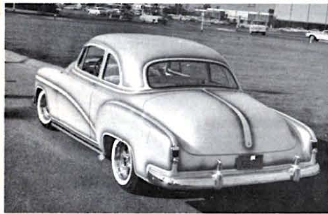
The '51 Chevy has pearl white exterior with blue trim. Same idea in colors extends to the interior tuck and roll upholstery and rugs. All body seams are filled.
