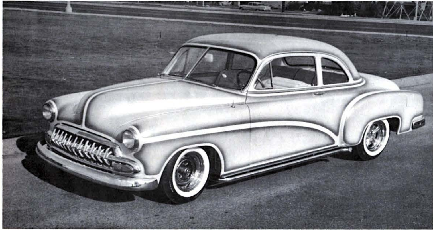
CHANGES INCLUDE '54 GRILL TEETH, MOLDED BUMPER, PEAKED HOOD, DECKED, NOSED AND ALL BODY SEAMS FILLED IN.
