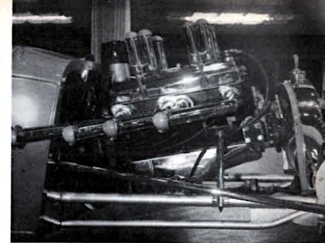
Three photos at left and above show '32-Austin-bodied red roadster of Skip Gibson, John Peterson and Mel Madison, all of Santa Maria, California. Engine 301 Chevy, with Thompson rods and pistons, Engle cam, B&M Hydra. Body is Cal Auto glass. Basic chassis is Lefty Mundersbach original, with coils at rear. New car has already turned 147.
