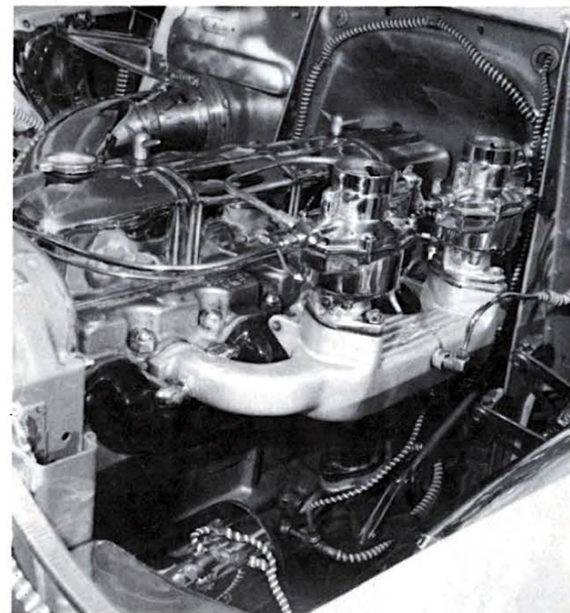
Engine is completely chromed. It is a '52 Chev, stock except for solid lifters and Isky three-quarter cam. The exhaust is porcelain covered. Carburetion has been improved.
