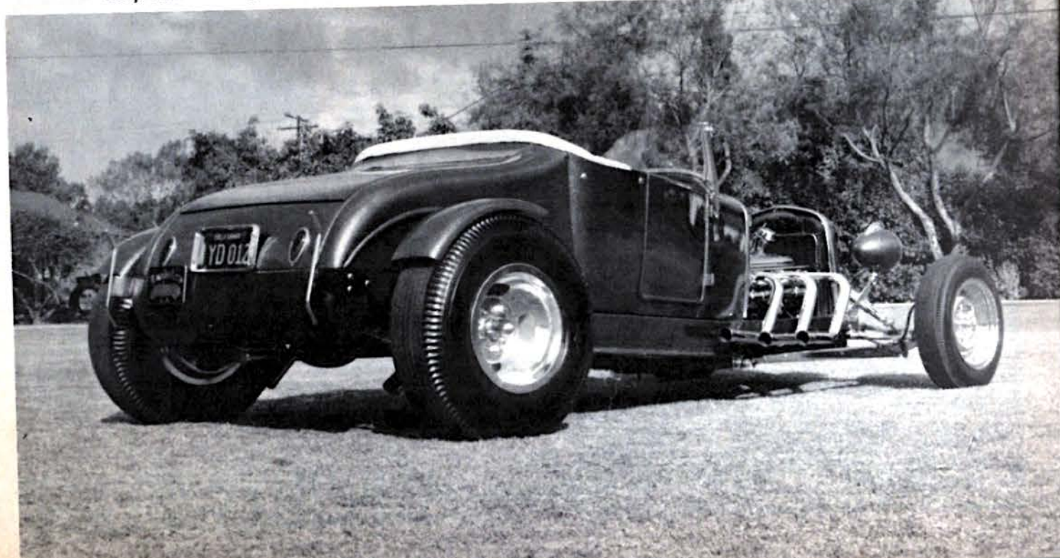
Red, white and chrome is the color scheme of this pure-bred roadster. Chromed aluminum rear wheels are originally from a truck design. Unique deep-dish steering wheel adds a different touch and allows better visibility.
