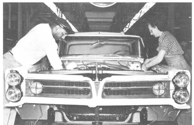
Following the installation of the hood, grille and front bumper, shown here, the car is thoroughly inspected and tested before being OK'd for shipment to the customer.
