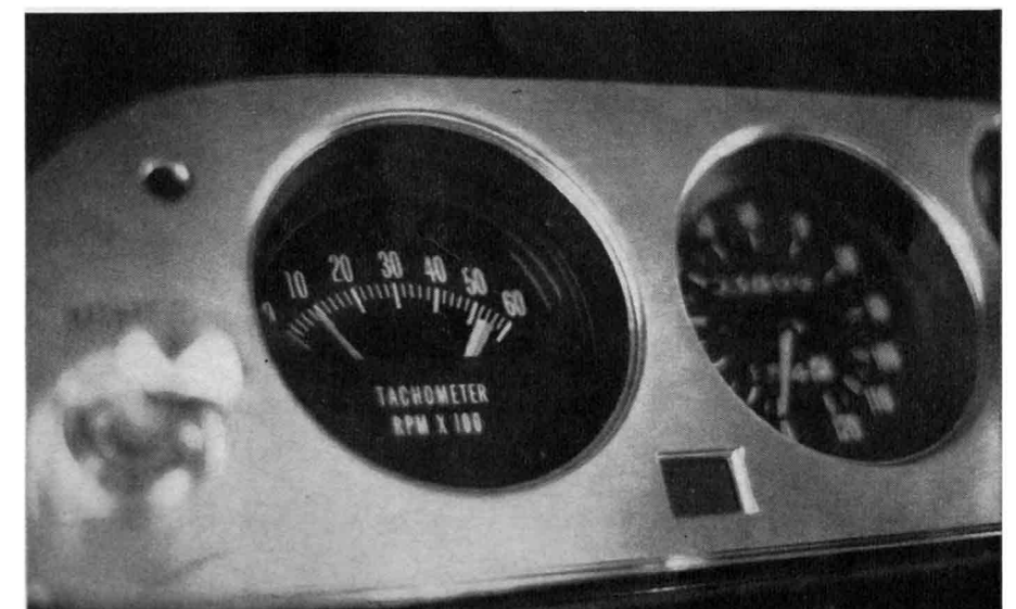
Brushed-aluminum dash is handsome, with nearly complete set of instruments, but markings on tach are too small for quick readings; full-circle dial would help.
