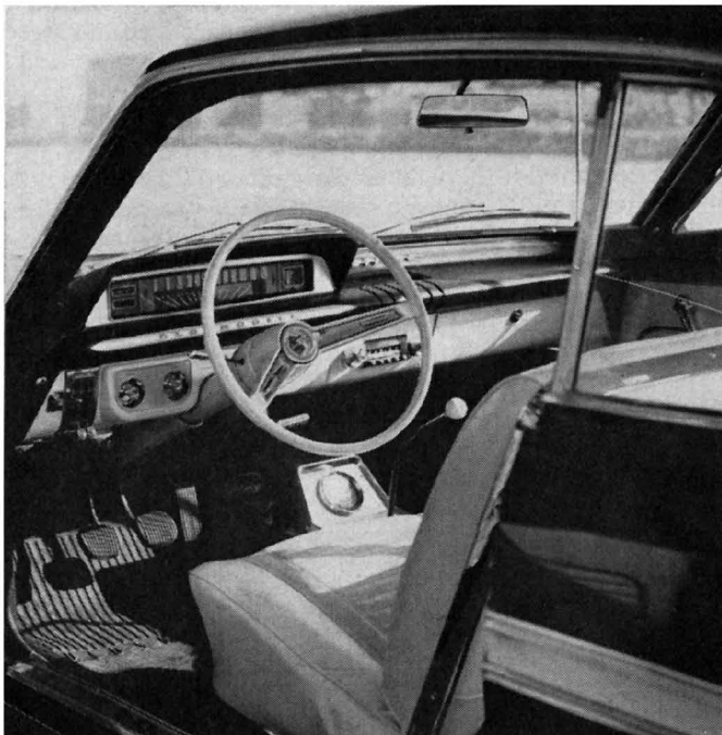
Driving position is sensibly low with no offset on steering wheel or pedals, the driver facing exact direction of travel.
