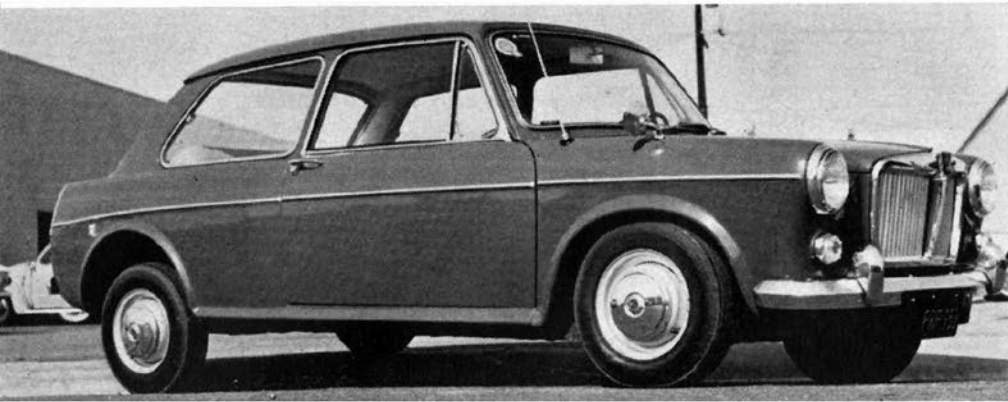
BODY REMAINS LEVEL although far side rear wheel is on curb and near wheel is in gutter.
