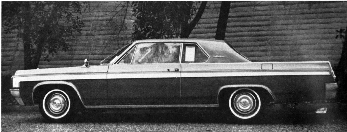
WIDE ALUMINUM strip is exclusive trim. Starfire shares roof and concave rear window with only one other GM car.
