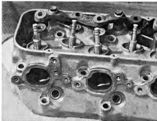
Minus springs, it's easy to see how valves are angled to favor port supplying them and also to open away from walls. Note cast pushrod guides.
