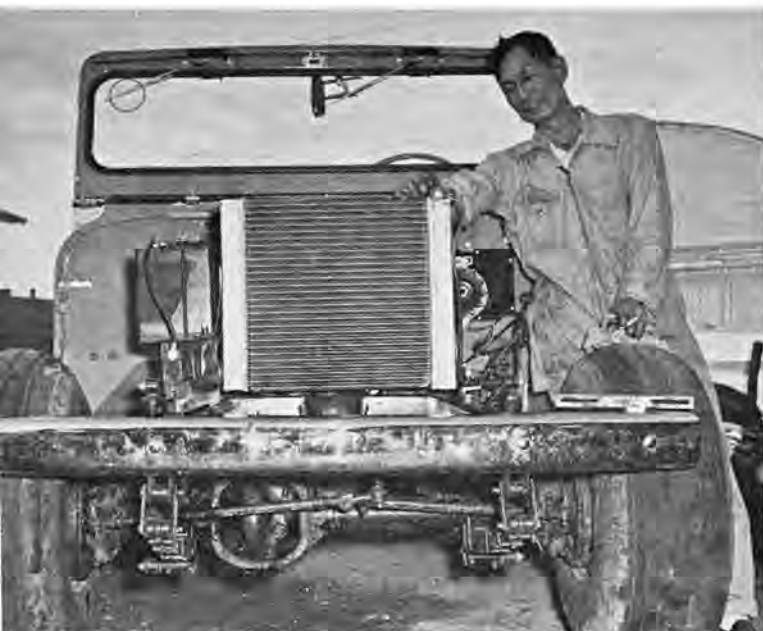
The radiator was built by Dyke Kagihara, left, who runs a radiator repair shop in Honolulu. As the radiator cooled the Chevy without any problems, Dyke had reason to be proud of his work. With the exception of the steering gear and its linkage, shown at right, a Jeep engine compartment has enough room for almost any automobile-type V8. Because of the way it is mounted, the steering gear is difficult to move. For the Chevy installation the engine was moved instead and the oil filter left off.
