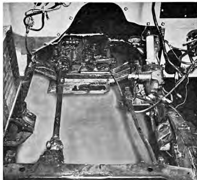
The radiator was built by Dyke Kagihara, left, who runs a radiator repair shop in Honolulu. As the radiator cooled the Chevy without any problems, Dyke had reason to be proud of his work. With the exception of the steering gear and its linkage, shown at right, a Jeep engine compartment has enough room for almost any automobile-type V8. Because of the way it is mounted, the steering gear is difficult to move. For the Chevy installation the engine was moved instead and the oil filter left off.
