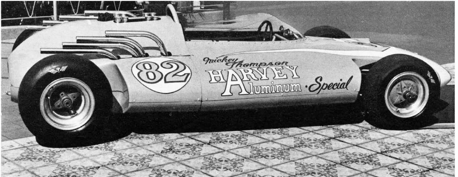
BARELY 21 in. tall at the cowl, the Thompson/Harvey Indianapolis Special has 12-in.-diameter wheels.
