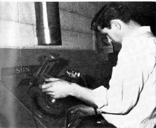
DISTRIBUTOR advance is altered.
