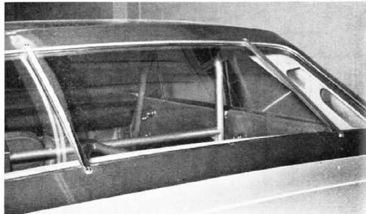
STEEL STRAPS on back window prevent "popping out."
