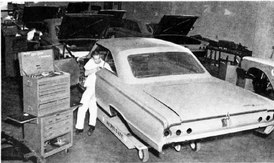
BODY SHOP scene: all cars are stripped, rebuilt and repainted to racing specifications.
