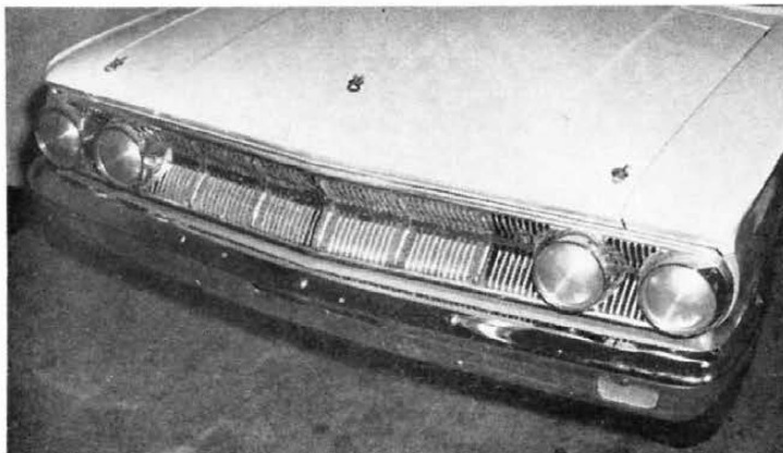
SAFETY PINS replace hood straps, prevent hood from flying off at high speed.
