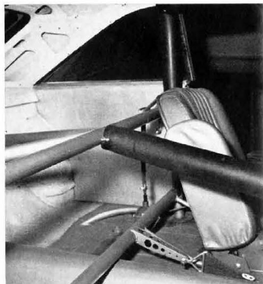
ROLL CAGE inside cockpit is constructed of 1.75 in. Shelby tubing; rubber wrapping protects driver. Below: tabs for door-bolts are welded in place.
