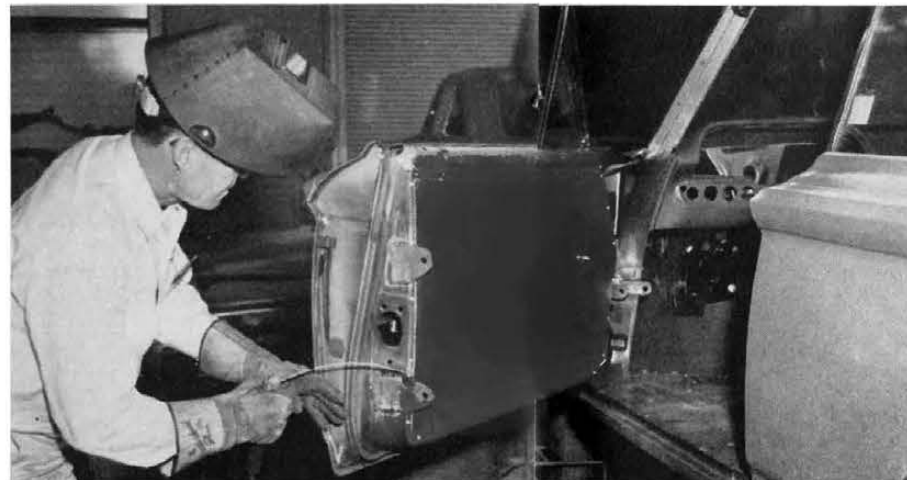
ROLL CAGE inside cockpit is constructed of 1.75 in. Shelby tubing; rubber wrapping protects driver. Below: tabs for door-bolts are welded in place.
