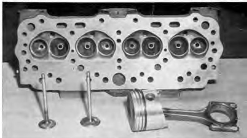
ABOVE—R3 cylinder heads are special castings with large ports and oversize valves. Chambers are machined, then polished. Valves are undercut, polished.
