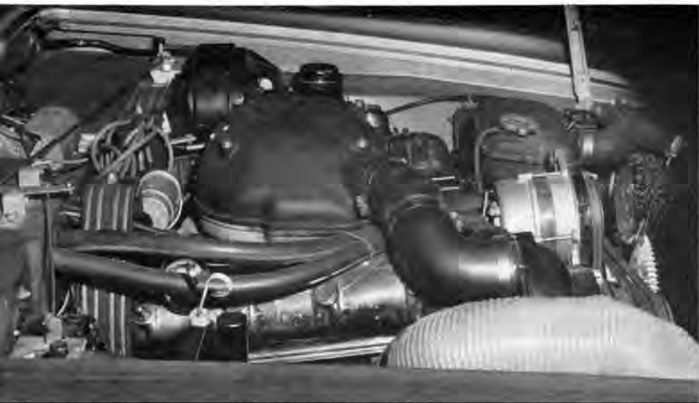
LEFT - The R3 engine uses a cast aluminum enclosure for the four-barrel carburetor instead of the stamped steel bonnet as on the R2. This completely pressurizes the carburetor and prevents leaks. R2 uses less pressure so does not need cast box. RIGHT - Avanti bodies have a stamped steel roll bar which extends from the floor pan, acts as the window post, then goes across the underside of the fiberglass top. It is heavily padded and covered with vinyl. Rear windows swing out only.
