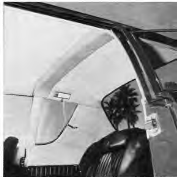
LEFT - The R3 engine uses a cast aluminum enclosure for the four-barrel carburetor instead of the stamped steel bonnet as on the R2. This completely pressurizes the carburetor and prevents leaks. R2 uses less pressure so does not need cast box. RIGHT - Avanti bodies have a stamped steel roll bar which extends from the floor pan, acts as the window post, then goes across the underside of the fiberglass top. It is heavily padded and covered with vinyl. Rear windows swing out only.
