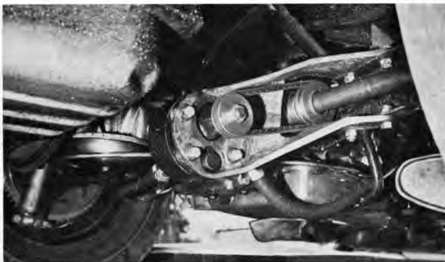
Nichels' mechanics attached an aluminum bracket to rear A-frame, then mounted a power steering pump with belt drive from pulley on right swing axle to circulate oil between transaxle unit and radiator. Undercar fuel tank has large notch in front to make room for the extra length of clutch assembly and throwout slave.
