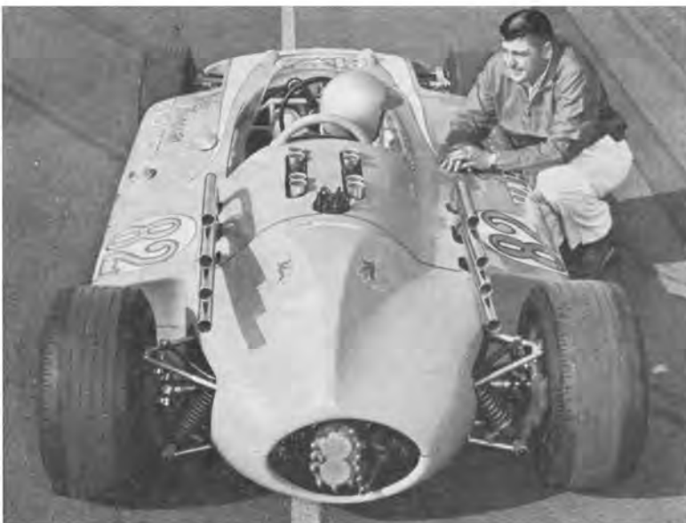
Mickey confers with Billy Krause after a test run. Air turbulence is minimized by extending body to fill space between wheels. Fuel is on left, right compartment is empty except for small oil cooler and its air duct. Tires are 7 inches wide front, and 9 inches wide at rear. Track width is 55 inches.
