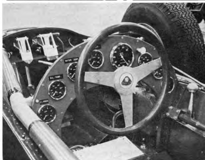
UPPER - Left to right: Jim Clark, driver of the second car; Dan Gurney, idea man behind the project; and Colin Chapman, builder of Lotus Grand Prix cars, in a pensive moment. LOWER - Well-filled dash panel becomes a structural bulkhead in monocoque construction. Driver will be too busy to monitor all these instruments. Steering is rack and pinion with 2\frac{1}{4} turns lock to lock of the light alloy 12-inch wheel.
