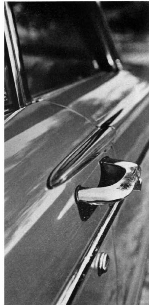
FALCON DOORS fit Comet with hastily attached rib.
