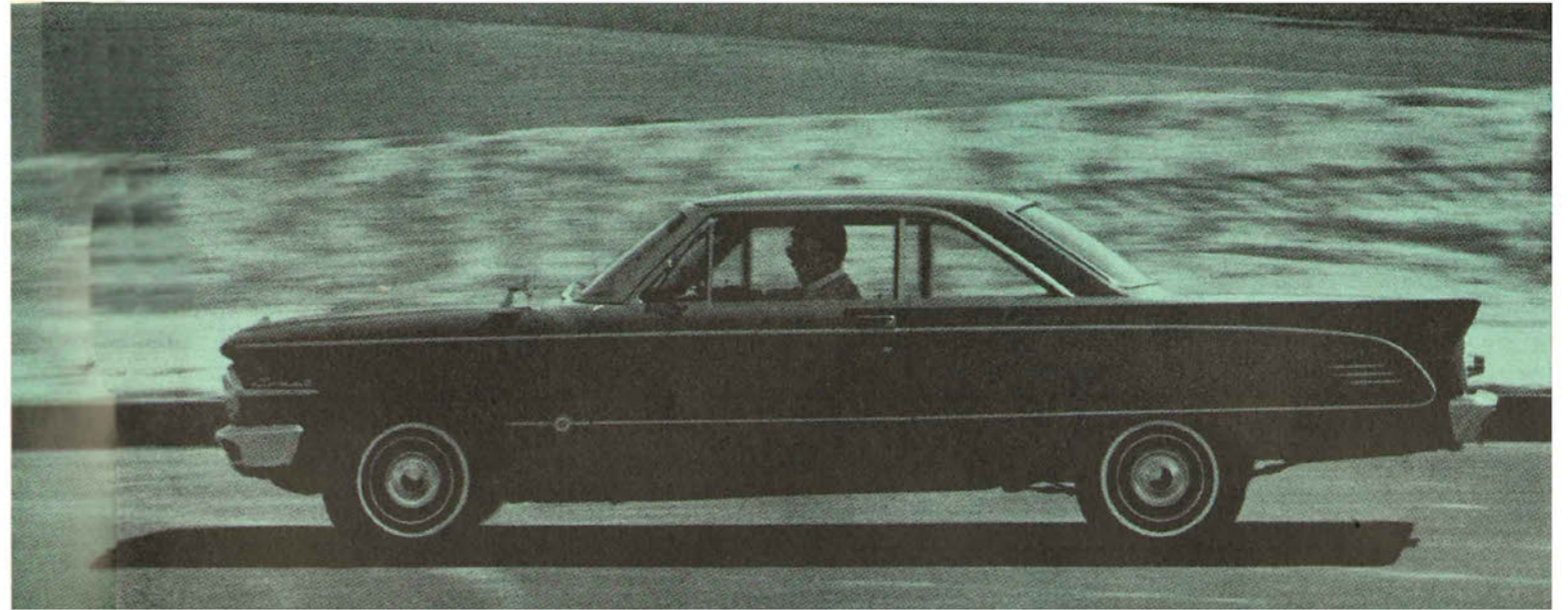
NEW CORNERING stability is shown in sequence of Comet Sportster, illustrating reduced body lean resulting from stiffer suspension. Sloping roofline is also shown to advantage.
