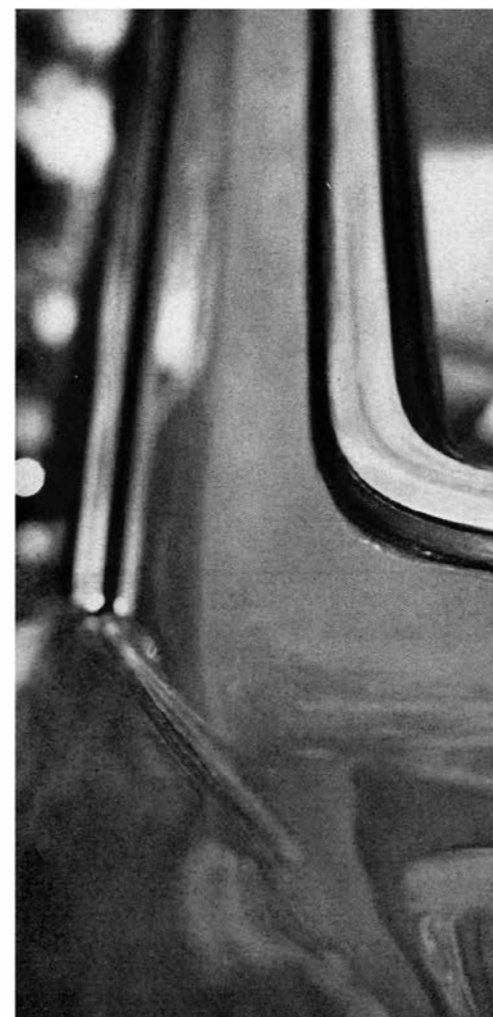
SLANTBACK roofline was marred by flaking paint over weld.
