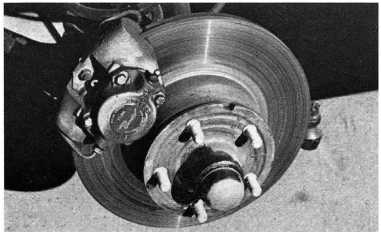
AVANTI DISC brake pads pinch against plate.
