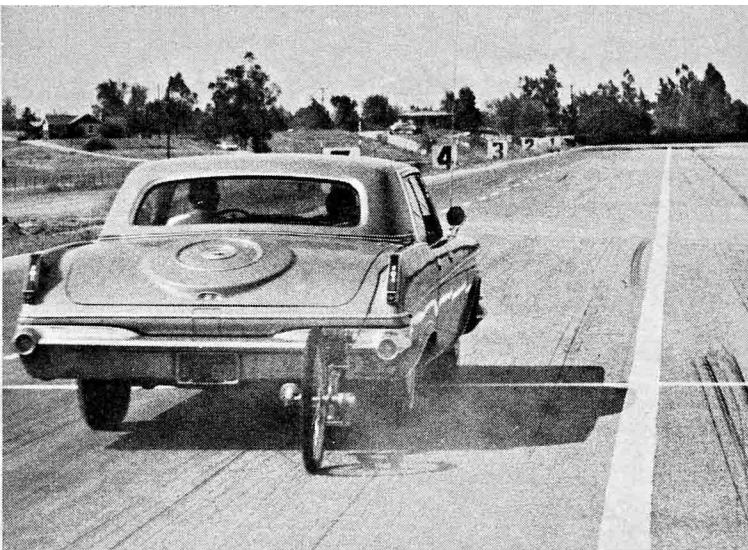
A single-diaphragm, vacuum-suspended power brake unit is used on new Imperials. It's easier to take apart or service and is built stronger than the dual-diaphragm unit used last year. Normal stops required only light pedal pressures, but we did notice considerable fade during stops from our high-speed and acceleration runs. Panic stops from 60 mph required longer-than-average distances for a car of this size and weight.
